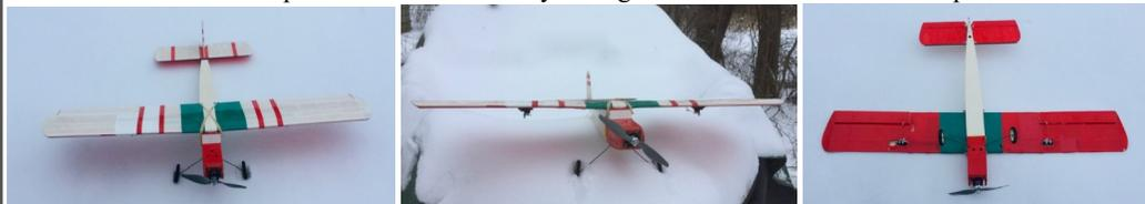
This is light weight 9 & 1/2 ounce Balsa and film covered flyer. The wingspan is 35&3/4", Overall length is 25". It has a Hacker motor with matching ECS and a 7X5 propeller. The 4 servos and motor work as expected and has 2" wheels. The tail wheel will have to be added. This should be a very good light wind flyer.
