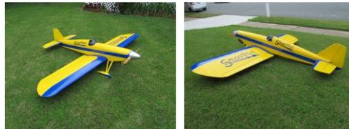
It is the Balsa USA Smoothie XL. The wing span is 88" and the fuse is 70" long. I haven't weighed it yet, maybe later today after I balance it. It has an RCGF 32" gas engine for power.
